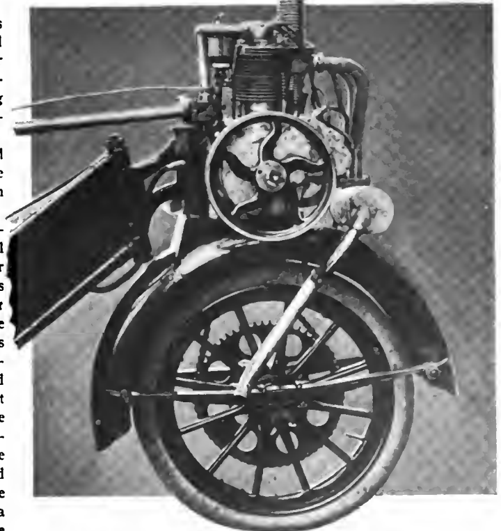
Power plant of the Maxim machine, showing motor mounting
